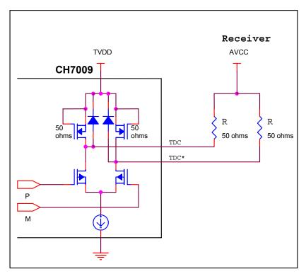
Figure 1: The simplified schematic of CH7009 DVI Output
