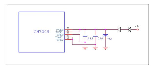
Figure 2: Isolate the CH7009 family TVDD power with a low forward-voltage diode (such as 1N5817)
