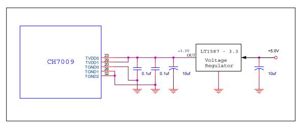
Figure 4: The circuit isolates the CH7009 TVDD power with a 5.0V - 3.3V voltage regulator
